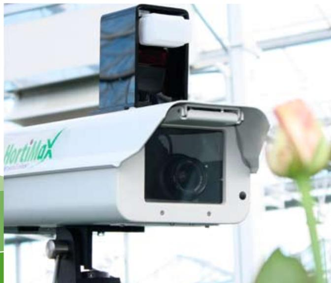
**CropView is a unique solution that allows you to keep track of your crop's development. CropView combines modern digital photography and computerised environmental control, so you can analyse both your crop's current condition and its growth over time. This is all done in unrivalled detail, and available whenever and wherever you want. In-depth field tests have already shown that CropView can result in substantial cost savings in both ornamental and vegetable production.**
